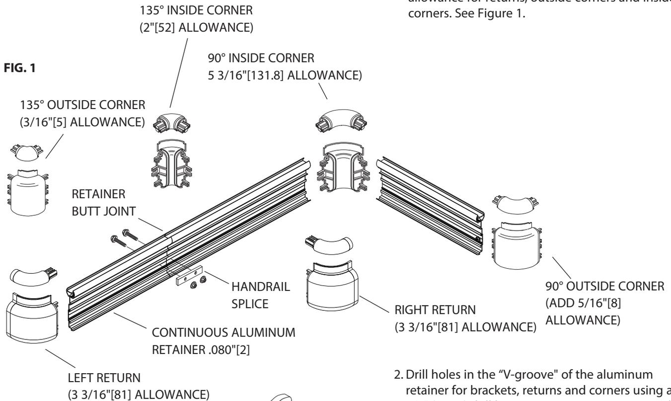
2. Drill holes in the "V-groove" of the aluminum retainer for brackets, returns and corners using a 1/4" (6mm) drill bit. Position retainer against wall at desired height allowing for returns and corners. When assembled, the top of the handrail is 4 1/16" [103] above the "V-groove." Level and mark bracket holes on wall. Drill marked holes with 3/4" (19mm) drill bit for toggle bolts (drywall installation) or 1/2" (13mm) drill bit for lead anchor (concrete wall application). See Figure 2.
